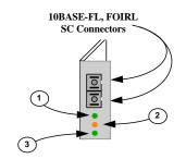
an SC-type "snap-in" connector instead of an ST-type "twist-lock" connector. Please refer to Section 3.2.4. for details.
